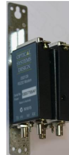
Figure 26 – OSD139 Fibre Optic Modem Bracket (FP1032) with two OSD139 modems
