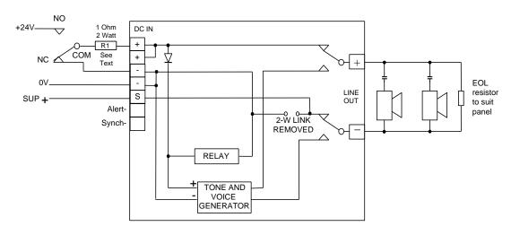
Fig 2 Mini-Gen Mk2 Connection With Separate Supervision (single pole / 4 wire)
