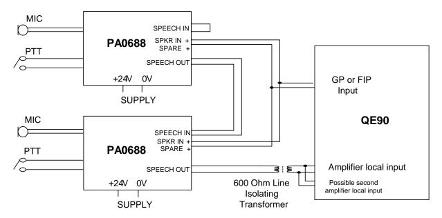
Figure 2 - Using PA0688 Pre-amp with QE90 Local Inputs
