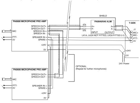
Figure 7 - Remote Emergency Microphone(s) for T-GEN 50
