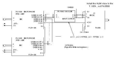
Figure 6 - Balanced Configuration, PA0688 to T-GEN 50, Non-emergency Microphone
