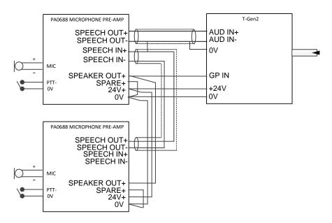
Figure 4 - Microphone Pre-Amp to T-Gen2
