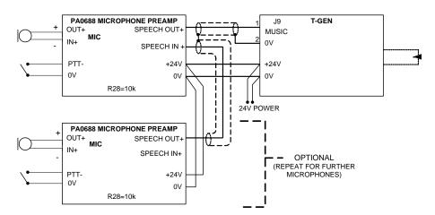
Figure 5 - Unbalanced Configuration, PA0688 to T-GEN 50, Non-emergency Microphone
