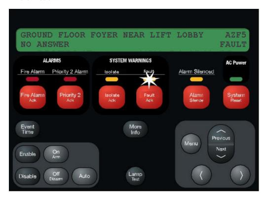
Figure 3-1. Operator Interface Showing Fault Condition
