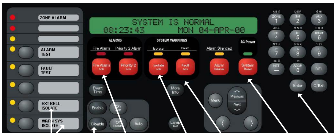
OUTPUT ISOLATES DISABLE FIRE ALARM ACK ISOLATE ACK FAULT ACK SYSTEM RESET ENTER
