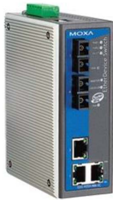
SU0319/SU0320 5 Port MOXA Switch
