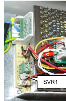
Figure 3-3 SVR1 location on PSU
