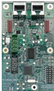
Figure 8-14 – MX1 Fan Control Expansion Kit
