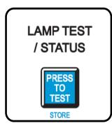
Press and hold the **LAMP TEST** key. All indicators will light up, all digits will read "8"s, and all but 8 decimal points will light. The normal display resumes when **LAMP TEST** is released.
