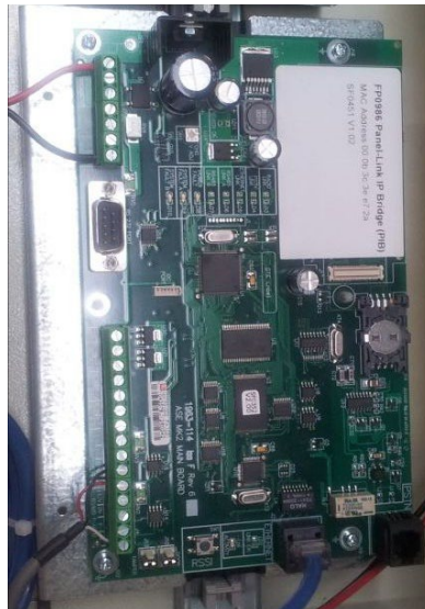
Figure 4-1 – FP1011 Bracket Holding PIB in QE90
