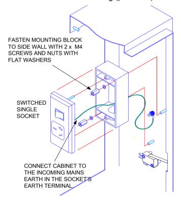
Figure 1 – Mains Outlet Location in MX1 Slimline Cabinet
