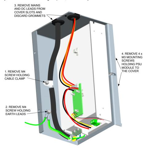
Figure 2 – Power Supply Preparation by Removing the Cover
