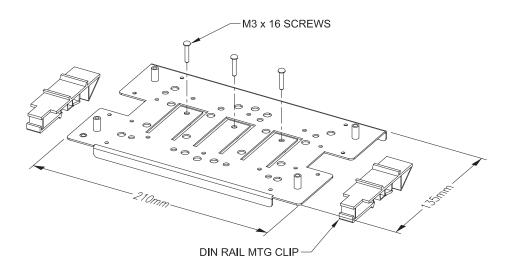
Figure 1 – (FP1011) DIN Rail Mounting Plate – Basic Assembly
