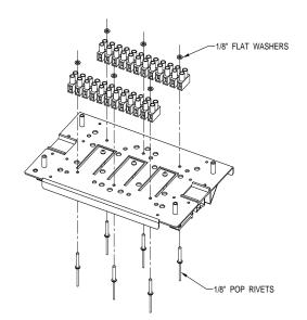
Figure 7 12 -way Terminal Block Mounting Method
