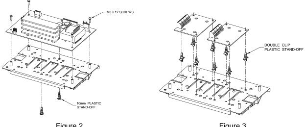
Figure 2 T-GEN, Responder, F3200 8 Zone Module, ASE Mk2/PIB Mounting Method
