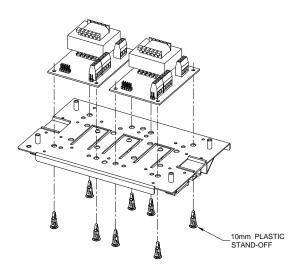
Figure 4 Mini-Gen Mounting Method
