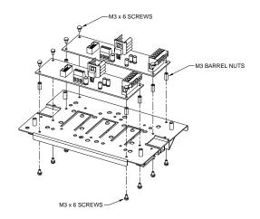
Figure 5 RS485 Board Mounting Method
