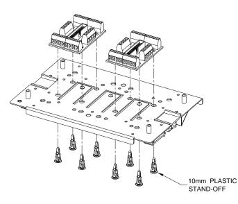
Figure 6 (Unprotected) Termination Board Mounting Method
