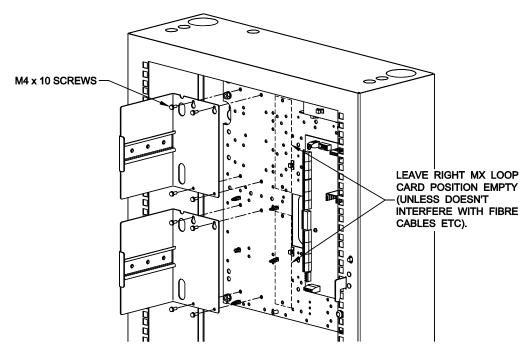
Figure 1 – FP1012 Bracket Mounting Positions on 15U Gear Plate
