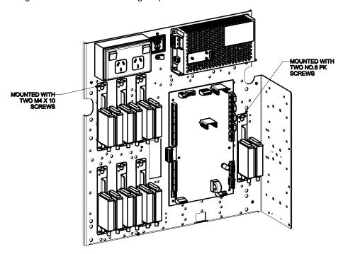
Figure 2 – FP1032 Bracket Mounting Positions on a 15U MX1 Gear Plate
