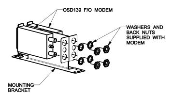
Figure 1 – Mounting OSD139 Modems on FP1032 Bracket
