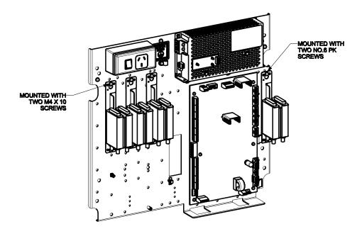
Figure 3 – FP1032 Bracket Mounting Positions on an 8U MX1 Gear Plate
