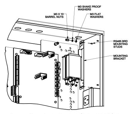
Figure 4 – FP1032 Bracket Mounting in Slimline MX1-NZ Cabinet
