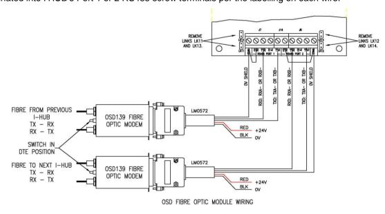
Figure 5 - Wiring of I-HUB RS485 Ports to OSD139 Modems
