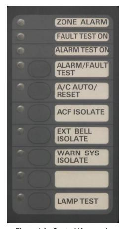
Figure 1-3. Control Keys and Indicators
