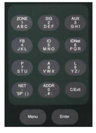
Figure 4-1. Function/Numeric Keypad
