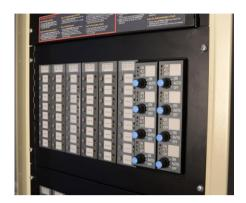
The display door mounts directly to the rack cabinet, and does not require an equipment bay for support. Any equipment bays in the cabinet must be mounted on the rear wall of the cabinet. This display door will not fit with equipment bays mounted to the front of the cabinet.
