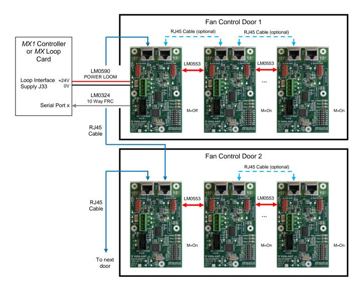
Figure 4 – MX1 Fan Control Boards Wiring Diagram
