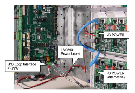
Figure 7 – Power Wiring
