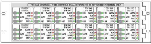
Figure 1 – MX1 Fan Control Door
