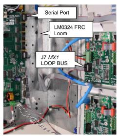
Figure 6 - Serial Port Wiring
