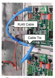
Figure 9 – Wiring multiple doors
