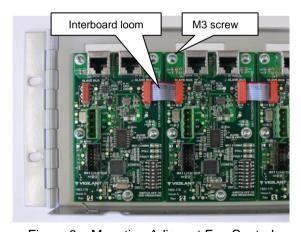
Figure 8 – Mounting Adjacent Fan Control Boards
