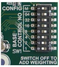
Figure 10 – DIP Switch Setting (Master and base control no = 7)
