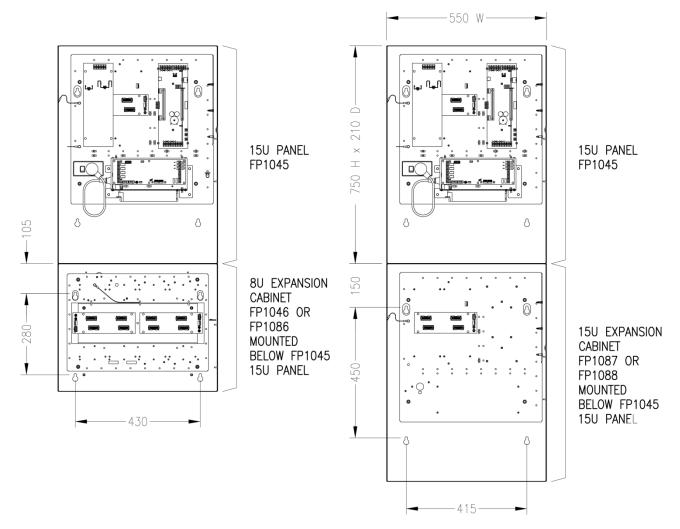
Figure 19. Mounting cabinets side by side
