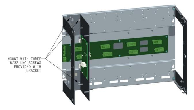
Mount the 4100-6072/6073 SM Fibre Modems on the left side of the expansion bay for best packing of the equipment.
