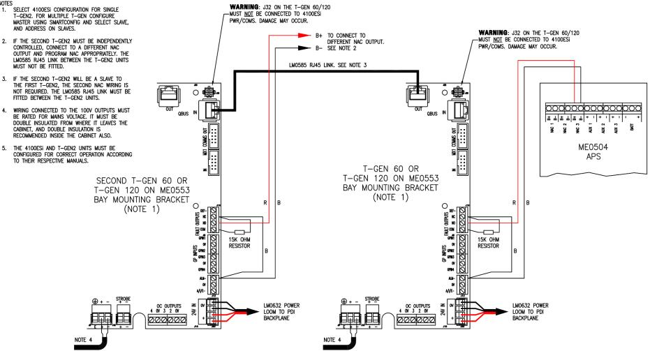
Figure 46. Wiring for T-GEN 60 and T-GEN 120 with switching modules
