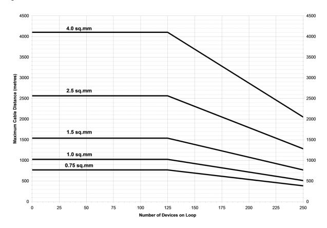
Figure 64. IDNet cable distance and device limits for common cable sizes
