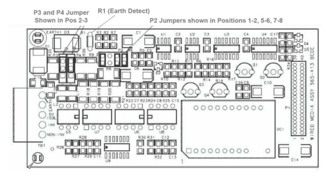
**P2**: Selects the wire type. Fit positions 1-2, 5-6, and 7-8 for  $1.0 \text{ mm}^2$  or heavier paired wiring. Remove all jumpers for twisted pair telephone cable wiring.
