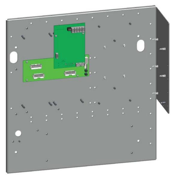
Figure 7. PDI card mounted on backplane in the 15U cabinet
