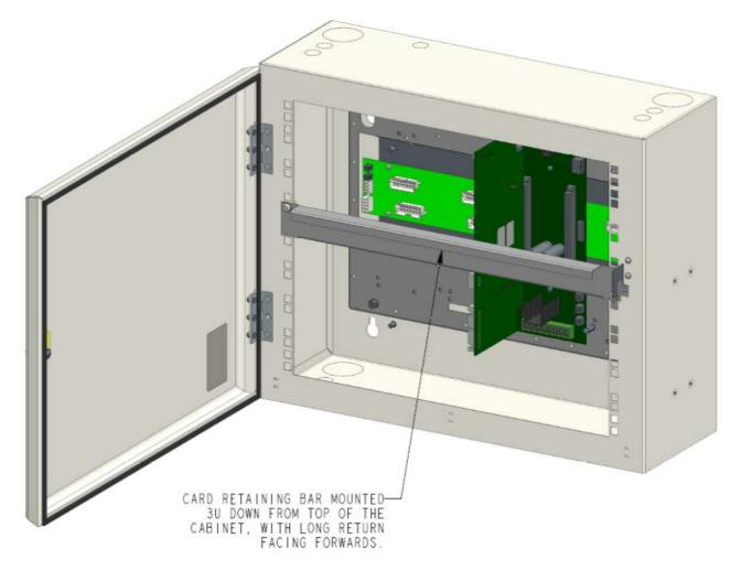
Figure 25. Legacy card retaining bar in the 15U cabinet
