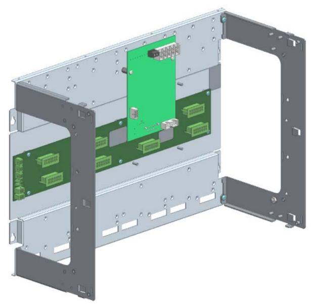
The bay back planes are linked together with compatible four-way looms distributing power and communications.
