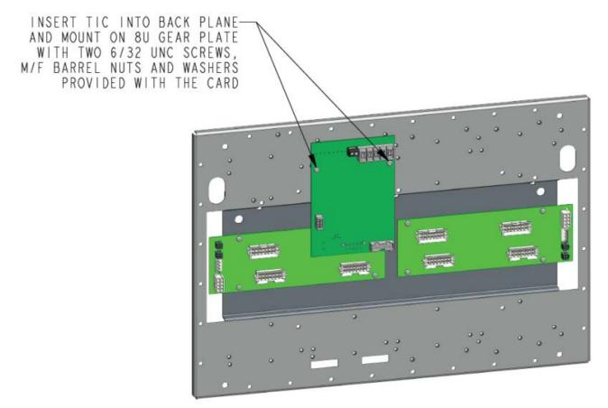
Plug the card into the socket on the backplane, and secure it with the two screws supplied with the card. The card draws power and communications from the PDI backplane. For information about field wiring, refer to *LTO432 Field Wiring Diagrams*.
