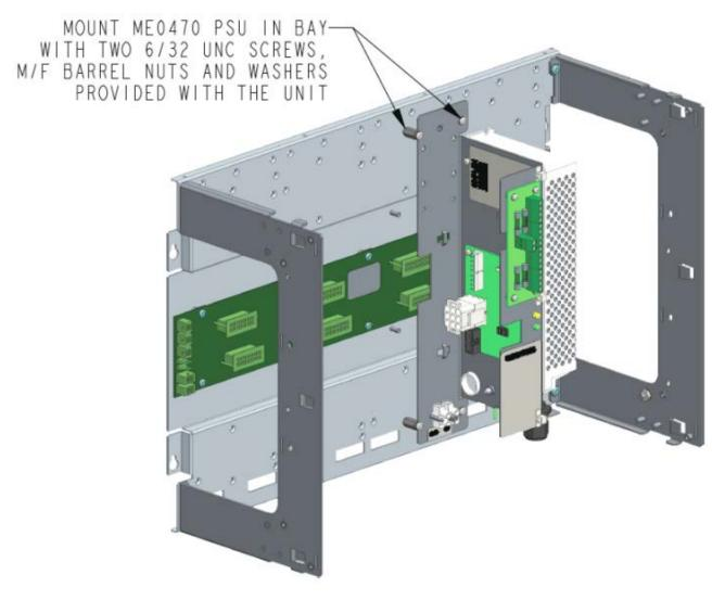
For information about configuring the ME0470 and for connection to the 4100ESi, refer to *LT0432 4100ESi Field Wiring Manual* drawings 702 and 705.
