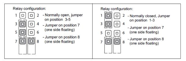
Leave circuits that are not used unprogrammed in the 4100ESi Programmer (Device Type = None). Set the links for Class B Conventional detector mode with no EOL fitted.
