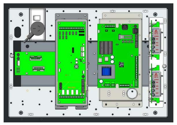
Figure 26. T-GEN 60 and 100 V Switching Modules in 8U cabinet with APS
