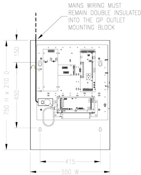
AS1670.1 requires a clear space of 1 m in front, and 0.5 m on each side of all cabinets that are to be used by emergency personnel. AS 1670.1 requires that the main touchscreen display (FBP), and all fan controls are between 750 mm and 1850 mm above the floor.
