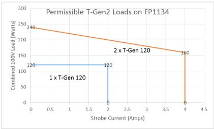
Figure 7 - FP1134 T-Gen2 100V Load vs Strobe Current
