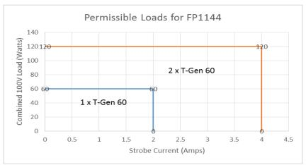
Figure 6 - FP1144 T-Gen2 100V Load vs Strobe Current
