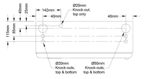
Figure 2 – 8U /15U Cabinet Cable Knockouts
