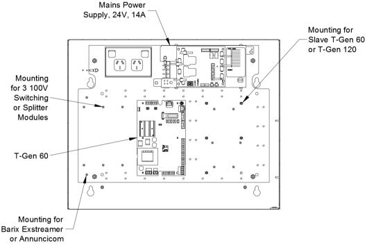
Figure 4 – 8U Gearplate Module Mounting Positions
