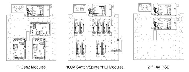
Figure 5 –15U Gearplate Module Mounting Positions
