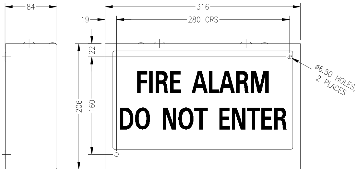
Figure 8 – AVI Mk2 mounting hole pattern.
