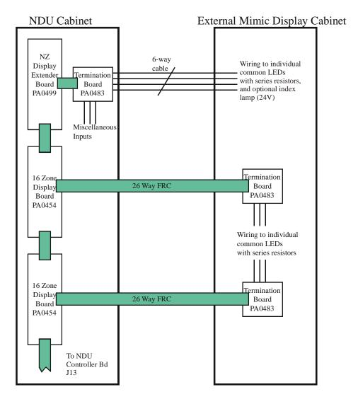
Note: PA0769 Termination Board can be used instead of PA0483 PA0769 has resistors for LEDs already fitted to the PCB.
