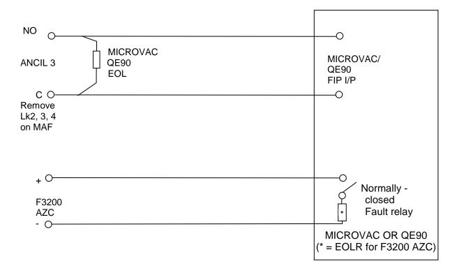
FIG 5.5.4 WIRING ANCIL 3 AND 8ZM INPUT TO MICROVAC/QE90
