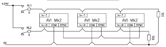
For FIRE ALARM / DO NOT ENTER, FIRE ALARM / EVACUATE AREA EOL = 2k7
