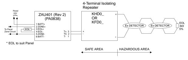
FIG 6.4.3.3 F3200 WITH ZAU401 & 4 TERMINAL IS REPEATER
