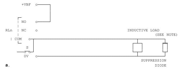
Note: For a load of less than 400 Ohms a diode of suitable current rating must be wired in series with the load at the load as shown in b. below.
