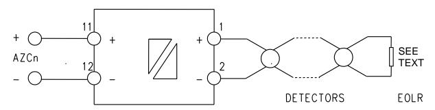
FIG 6.4.3.4 SHORT-CIRCUITING DETECTORS WITH 4 TERMINAL REPEATER
