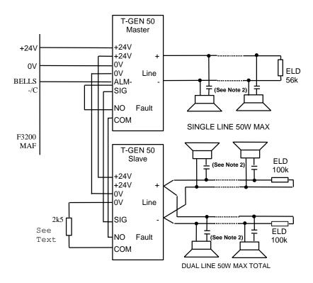
FIGURE 5.5.6 WIRING T-GEN 50 TO F3200 BELLS/ANC 3 RELAY
