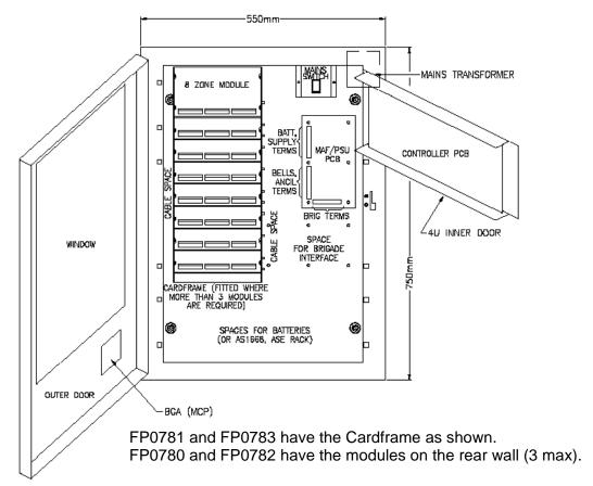
FIG 2.2.1 F3200 STANDARD CABINET WITH CARDFRAME - INTERNAL LAYOUT
