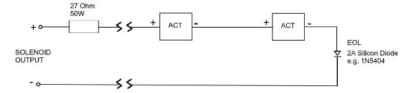
c) Multiple devices with limiting resistor (not recommended method).
