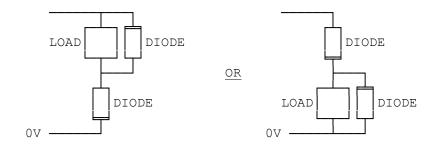
FIG 5.4.2 EXAMPLE OF PLANT RELAY WIRING WITH SUPERVISION
