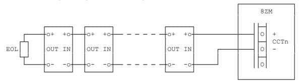
FIG 5.3.1 CORRECT AZC DETECTOR WIRING
