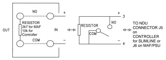
FIG 5.10.1 MCP CONNECTION FOR NDU, AUSTRALIAN MODE
