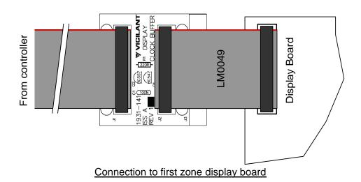
FIG 5.1.4 CONNECTION OF DISPLAY CLOCK BUFFER BOARD
