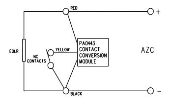
FIG 6.5.1 NORMALLY CLOSED CONTACT WIRING TO F3200 AZC
