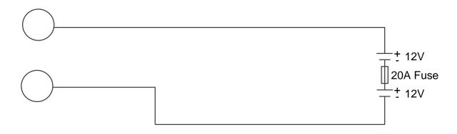
FIG 4.3.2 BATTERY OVERCURRENT PROTECTION FOR LOADS GREATER THAN 3A
