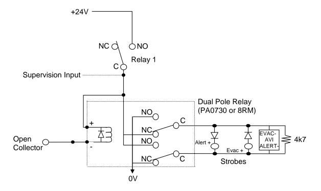
FIGURE 5.6.2 DUAL POLARITY OUTPUT FOR STROBES/AVI
