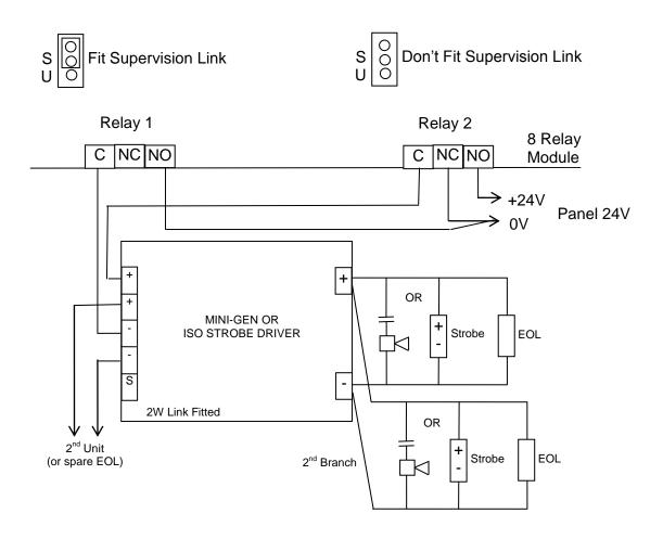
FIG 5.6.5 USING 2 RELAYS WITH 1/2 MINI-GEN/STROBE DRIVERS
