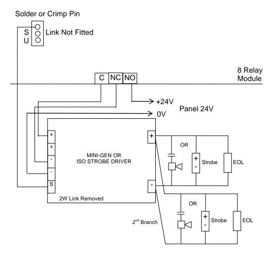
FIG 5.6.3 USING 1 RELAY OUTPUT WITH 1 MINI-GEN/STROBE DRIVER IN 4-WIRE MODE
