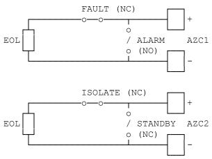
FIG 6.3.1 EXAMPLE OF SUB-FIP MONITORING USING 2 AZCS
