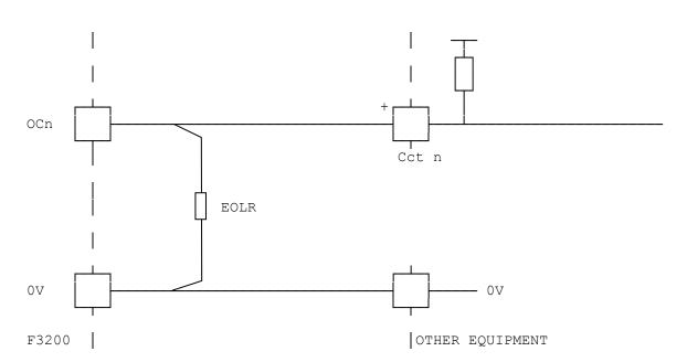
FIG 5.7.2 EXAMPLE OF INTERFACING TO OTHER EQUIPMENT, DIRECT COUPLING
