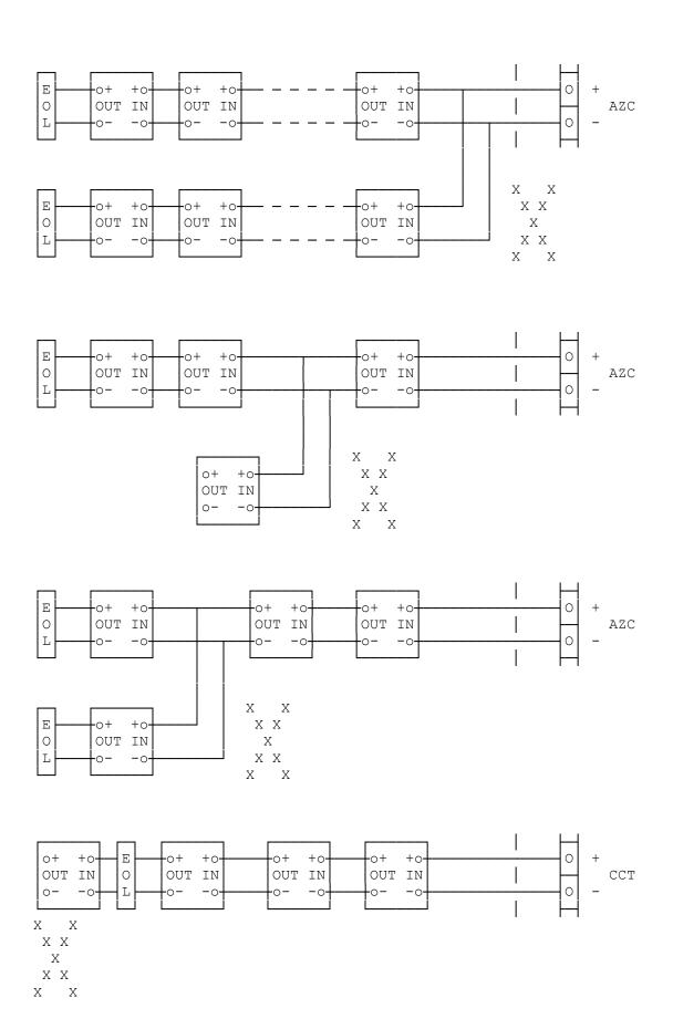
FIG 5.3.3 EXAMPLES OF INCORRECT AZC WIRING
