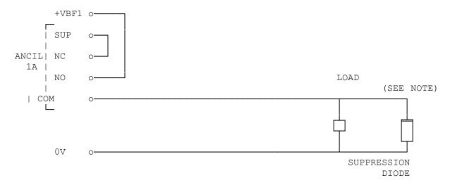
Note: For a load of less than 400 Ohms a diode of suitable current rating must be added in series with the load at the load as shown below.
