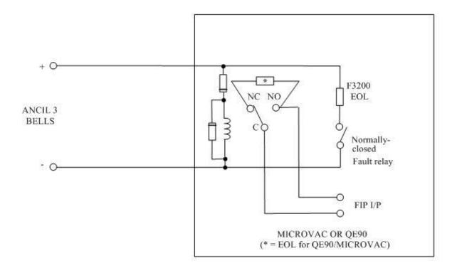
FIG 5.5.3 WIRING ANCIL 3 TO MICROVAC/QE90
