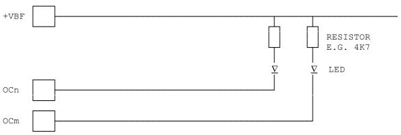
FIG 5.7.1 EXAMPLE OF LED MIMIC WIRING
