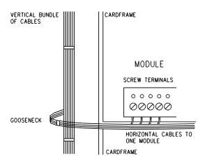
FIG 5.2.2 GOOSENECK CABLING
