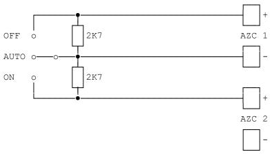
FIG 6.1.4 FAN CONTROL WITH TWO AZCs & ROTARY (OR CENTRE-OFF) SWITCH
