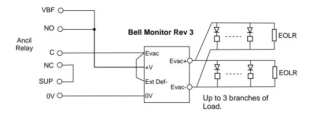
FIGURE 5.4.3 <u>EXAMPLE OF SUPERVISING MULTIPLE BRANCHES OF MULTIPLE LOADS</u>
