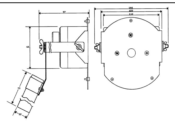
Fig. 2 T110 Test Source - Overall Dimensions
