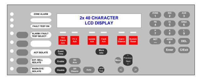
0-5-13 Fault Test Active LED (P515)
