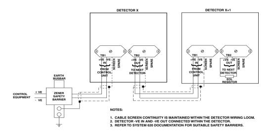
Fig. 5 Detector Wiring - Intrinsically Safe Circuits
