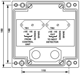
Fig. 2 Fixing Dimensions
