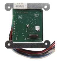
SIMPLEX AMZs provide an accurate, multi-featured 4-20mA interface for connecting analog sensors to Simplex addressable fire detection panels. The panel monitors the sensor and annunciates whenever a selected threshold level or fault condition is observed. Typical applications include: gas, air, liquid temperature, humidity, and air velocity sensing. The maximum distance from AMZ to a sensor is 1km. Each AMZ requires an address and up to 100 AMZs can be connected per panel.
