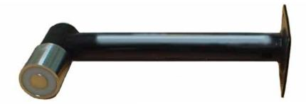
The EAO411 Electromagnetic Door Holder is designed to hold fire and smoke doors open under normal conditions, but automatically close under their own spring return mechanism when a fire or smoke alarm system is activated. The door is held open by the magnetic force
