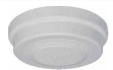
EA0031/33 are designed to mount directly to the underside of concrete slabs or inaccessible ceilings. The housing is surface mounted with concealed internal fixings. Speaker cable entry can be either from the rear, or via surface mounted conduit (four 19mm conduit knockouts are provided)
