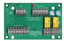
The MIO800 Multi-Input Output Module allows multiple input and output connections to be made between external equipment and the *MX DIGITAL* loop. Three inputs and two outputs are provided. Each input and output can be programmed independently to provide customised functionality.
