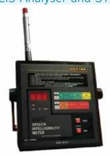
The STI-CIS Analyser measures the speech intelligibility of a fire alarm evacuation signal. To measure overall speech intelligibility, the STI-CIS Analyser uses the STI measurement method to factor in the effects of the warning system, room acoustics (reverberations and echoes) and background noise.
