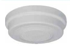
EA0029 is designed to mount directly to the underside of concrete slabs or inaccessible ceilings. The housing is surface mounted with concealed internal fixings. Speaker cable entry can be either from the rear, or via surface mounted conduit (four 19mm conduit knockouts are provided).
