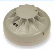
The 850H is a flexible cost-effective addressable heat detector with most of the features of MX VIRTUAL detectors. The 850H reports the temperature to the MX fire alarm panel which allows various detection modes. The 850H uses a high quality thermistor with very low thermal mass. This allows the detector to function as a heat detector as well as providing a fast and accurate temperature display.
