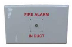
The E500 Mk2 range of remote indicators provide remote indication of an alarm condition on a fire detector. They are used where the fire detector is installed in an inaccessible location, and indication of alarm must be provided in an easily accessible area. For example, where the detectors are in roof spaces or cupboards, under the floor, or in hotel rooms, and indication is required in the room or corridor.
