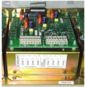
PA0795 TRAN9706-1 4x10W Transformer Module without Relays
