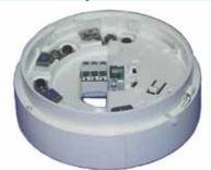
The 814RB Addressable Relay Base provides two sets of changeover volt-free relay contacts capable of switching 1A (resistive) @30Vdc. The relay function is controlled by the *MX* fire alarm panel via the detector fitted to the 814RB. The 814RB may be mounted to the ceiling, plugged into an M614/5B Universal Base or an 5BI/814IB Isolator Base.
