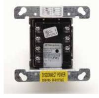
The 4090–9119 allows a 4100ES IDNet communication channel to monitor an unsupervised input contact with one point and control an output relay with the other point, yet occupy a single address. The input circuit and relay operation are controlled independently and may be disabled separately. Module power is supplied from the IDNet communications channel eliminating the need for separate power wiring. The address is set by DIP switch under the resealable label.
