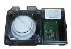
The TrueAlarm duct sampling unit detects the presence of smoke in air conditioning or ventilating ducts. Sampling tubes are installed into the duct and air is directed to a 4098-9714EA smoke sensor mounted in the housing.
