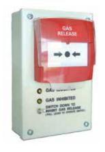
**FP0570** Local Gas Control Station - Automatic. Local Gas Control Stations (LGCS) are used in gaseous fire extinguishing systems to provide local area manual control of a release. The automatic version includes a Gas Inhibit switch, buzzer and LED, whereas the manual version (FP0572) does not. The LGCS is fitted with a resettable no-break plastic frangible element.
