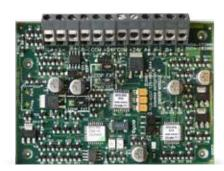
The DDM800 Detector Module designed to monitor and signal alarms from
