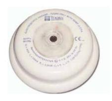
The 801FEx Intrinsically Safe Flame Detector forms part of the 800Fx Intrinsically Safe Series of MX Addressable Fire Detectors. The detector plugs into a 5BEx base. The detector is designed to transmit to a remote MX fire controller, digital signals which represent the infrared radiation produced by flaming fires involving carbonaceous materials. The 801FEx is a full featured flame detector for indoor applications. It must be connected via an EXI800 interface and galvanic barrier.
