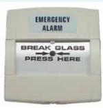
The SU0608 MCP is surface mounting, with a plastic coated glass element to ensure reliable, safe operation. It is coloured white (for EWIS applications) to be used where a fire alarm system does not exist. The call point is operated when the glass element is snapped, releasing the MCP's micro switch, which signals an alarm to the EWIS panel. The element is snapped by pressing on its centre - a hammer, or other impact device, is not required.
