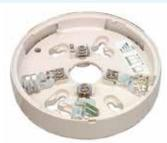
The **B501AUS** is a direct replacement for the Z131A Detector Base, and should be mounted on a flat surface with suitable fasteners. A tamperresist feature is incorporated in the base which, when used, prevents removal of the detector without using a small screwdriver or similar tool.
