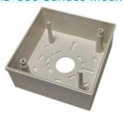
The SMB-500 provides mounting facilities for ADC/ADM/ADS130-Mk2 devices. The SMB-500 has mounting facilities for one of the above the modules and cover plate. The box may be secured to a wall with screws and plastic anchors (provided) or to a junction box (screws not provided).
