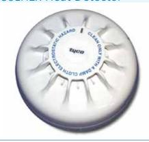
The 801HEx Intrinsically Safe Heat Detector forms part of the 800Ex Intrinsically Safe Series of MX Addressable Fire Detectors. The detector plugs into a 5BEx base. The detector is designed to transmit to a remote MX fire controller, digital signals which represent the status of the heat element of the detector. Software within the controller is used to interpret the returned heat values to raise an alarm or other appropriate response according to the programmed
