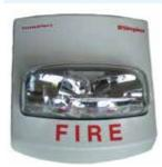
The 4906-910x Multi-Candela strobe is a high output xenon strobe capable of signalling evacuation using the ISO 8201 "T3" temporal pattern, as required by AS1670.4-2004 and AS 1670.1-2004. It produces white light with a link-selectable intensity of 15cd, 30cd, 75cd or 110cd. It is controlled by either the ISO 8201 Strobe Driver Module (PA1043) or a QE90 STRM Strobe Relay Module (PA0697)
