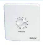
These 100V line audio attenuators install in a standard electrical flush box or mounting block. Screwdriver terminals enable a simple and neat connection. Models for 10W, 40W and 100W have an override relay facility. With fire evacuation systems it is necesary to override the attenuator setting to broadcast an announcement at full volume. The override relay requires 24Vdc to allow the attenuator to operate normally. This 24Vdc can be provided from the QE90 Amplifier Transformer Relay Output.
