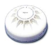
Where environmental conditions rule out the use of smoke detectors, MD601Ex/MD611Ex heat detectors may provide an acceptable, though less sensitive, alternative. For general use (particularly where the ambient temperature may be low) a 'Rate-of-Rise' (ROR) heat sensor is preferred. These detectors react to abnormally high rates of change of temperature and provide the fastest response over a wide range of ambient temperatures.
