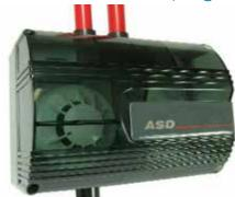
The ICAM IAS Air-Sampling Smoke Detection system provides a flexible detection solution to meet the needs of numerous applications. The IAS systems actively draws air from the protected area through sampling holes in a pipe network. Sampled air is filtered and then analysed by two *MX* detectors. The IAS system is available as a twin inlet pipe configuration (IAS-2), and can be fitted with two detectors per system. Flow failure is reported as a device fault via an MX MIM800 module.
