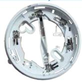
The 4B–C Continuity Base is used for most installations involving 850 Series detectors, as it allows the detector's in-built short circuit isolation function to be in-circuit when the detector is fitted and ensures continuity is maintained when the detector is removed. Use with MX1, 4100ESi.
