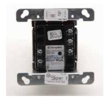
The 4090-9002 Relay IAM allows the CIE to control a remotely located Form "C" Relay contact using IDNet addressable communications for both data and module power. Typical applications are for switching local power for control functions such as magnetic door holders, or control of HVAC components, pressurisation fans, dampers, etc. Relay contact status is also communicated to the CIÉ. The address is set by DIP switch under the resealable label.
