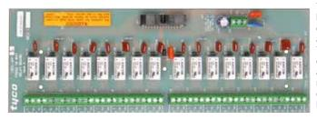
The 16-Way Relay Board has the same physical dimensions and footprint as the 32-Way Protected Termination Board, It comes complete with a 1.4 metre 26-way flat ribbon cable (LM0056) for connection to one of the IO-NET output connectors.
