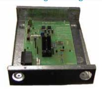
The IO-NET Programming Unit transfers the program to the IO-NET Controller PROMs. The Programming Unit is supplied complete with a cable to connect to a PC, the compiler programming software and the user manual. An external 24Vdc supply is required. IO-NET is also able to be programmed using SmartConfig Version 1.6 onwards. If the IO-NET site specific configuration is stored in read-only memory. It may be re-programmed multiple times before requiring replacement (SF0239).
