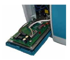
The VIO800 is an arrangement of the MIO800 Addressable Multi-I/O Module supplied ready to be fitted on to a VESDA LaserPLUS™ or Laser SCANNER The MIO800's inputs and outputs are wired to the relay outputs and control inputs of the LaserPLUS or Laser SCANNER to allow compatible MX CIE to monitor and control the VESDA units. Use with MX1, 4100ESi.
