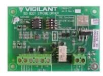
The ISO 8201 Strobe Driver generates an ISO 8201 compliant "T3" pattern for the Multi-Candela strobe 4906-9104.
