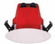
The 'One-Shot' PA speaker and grille is designed to install easily into 10 to 13mm gyprock/plaster/acoustic ceilings. Simply drill the required size hole, terminate the wiring and push the speaker into the ceiling until it snaps into place. They are designed to meet the requirements of AS ISO7240.24, with a cover and 22µF capacitor. The transformer has 5 power taps from 0.33 to 5W and a 4 way wireprotected terminal block.
