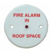
The E500 Mk2 range of remote indicators provide remote indication of an alarm condition on a fire detector. They are used where the fire detector is installed in an inaccessible location, and indication of alarm must be provided in an easily accessible area. For example, where the detectors are in roof spaces or cupboards, under the floor, or in hotel rooms, and indication is required in the room or corridor.
