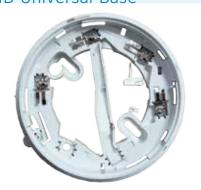
The 4B Universal Base contains no electronics and is suitable for indoor applications of the 614 series conventional (non-addressable), 814 and 850 series analogue addressable detectors. It provides excellent space for cable access and terminations. It features remote LED connections and an anti-tamper facility. The 4B base is designed to snap-fit into the ceiling tile adaptor, or screw fix to the ceiling in the traditional manner.
