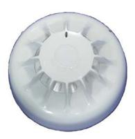
The 814H is a flexible cost-effective addressable heat detector with most of the features of MX VIRTUAL detectors. The 814H returns the temperature to the MX fire alarm panel which allows various detection modes, including all AS 1603.1 Types and many
