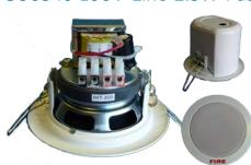
The SU0346 (HIT-300) is a 75mm fast-fit 100V Line Loudspeaker with a very low profile – only 70mm – which fits in most wall and ceiling cavities. It offers transformer-coupled 0.33W, 1.0W, and 2.5W power taps, plus an integral DC blocking capacitor. Spring-loaded clamps allow installation directly into an 86mm ceiling aperture without needing any other fixings. It offers clear sound reproduction of both emergency tones and voice messages.
