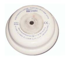
The 801FEx Intrinsically Safe Flame Detector forms part of the 800Ex Intrinsically Safe Series of MX Addressable Fire Detectors. The detector plugs into a 5BEx base. The detector is designed to transmit to a remote MX fire controller, digital signals which represent the infrared radiation produced by flaming fires involving carbonaceous materials. The 801FEx is a full featured flame detector for indoor applications. It must be connected via an EXI800 interface and galvanic barrier.
