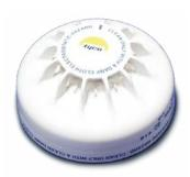
The MDU601EX detector combines the features of both the MU601EX detector and the MD601EX detector to provide a combined CO and Rate of Rise Heat Detector where the sensitivity of the CO detector is enhanced in response to a fast rate of change of temperature.
