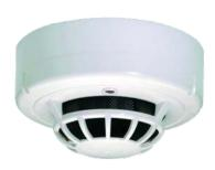
The 2351TEM photoelectric smoke/thermal detector incorporates an optical chamber and a thermal element, which in turn are continually monitored by an on board processor using algorithms developed specifically for the unit. An alarm signal is only enabled in the detector once the processor is satisfied that an incipient fire has been detected. By using a combination of inputs, the incidence of nuisance alarms is reduced while at the same time, the response time to an actual fire is also improved.
