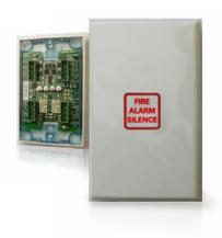
The AZM800 is a loop-powered MX Addressable module which cost-effectively integrates many of the key functions required for Type 5 fire alarm systems as defined in the NZ Building Code Compliance Documents, and in particular providing "hush"-able local alarm functions with brigade calling heat detectors and call points on the same circuit.
