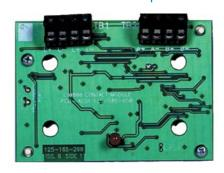
The CIM800 Addressable Contact Input Module monitors and supervises 2 circuits of voltage-free contacts such as outputs from extinguishing systems, ventilation controls, fire door controls, sprinkler flow switches, non-indicating hard contact detectors, etc. The LED illuminates when any input goes into alarm and can be
