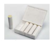
Part Number Ventilax Smoke Cartridge, 5 60g cartridges, dia 18x62mm, 17m<sup>3</sup> smoke vol, 180-240s burn time
