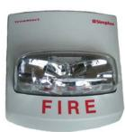
The 4906-910x Multi-Candela strobes are high output xenon strobes capable of signalling evacuation using the ISO 8201 "T3" temporal pattern, as required by AS1670.4-2004 and AS 1670.1-2004. They produce white light with a link-selectable intensity of 15cd, 30cd, 75cd or 110cd. Control is by either the ISO 8201 Strobe Driver Module (PA1043) or a QE90 STRM Strobe Relay Module (PA0697).
