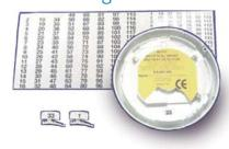
The 800 Series detectors incorporate a feature which automatically transfers the address flag to the detector base when the detector is plugged into the base. On removal of the detector the address flag is retained in the base, thus helping to ensure that detectors are not accidentally returned to the wrong detector base following service routines. Address flags are supplied in packs of 100.
