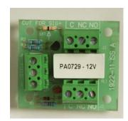
12V (PA0729) and 24V (PA0730) versions of a two pole changeover contact general purpose relay board may be used in either of two modes:
