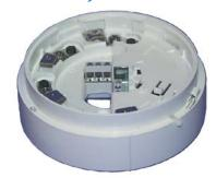
The 814RB Addressable Relay Base provides two sets of changeover volt-free relay contacts capable of switching 1A (resistive) @30Vdc. The relay function is controlled by the *MX* fire alarm panel via the detector fitted to the 814RB. The 814RB may be mounted directly to the ceiling or plugged into a 4B/5B, Universal or 4B-I/5B-I Isolator Base.
