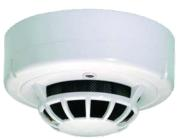
The 5351E thermal detector incorporates an Application Specific Integrated Circuit (ASIC). Combined with the latest in thermal element technology the detector provides efficient and accurate detection of fires, especially in environments such as bars or kitchens where smoke detectors are inappropriate due to the high level of airborne contamination.
