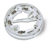
The 4B Universal Base contains no electronics and is suitable for indoor applications of the 614 series conventional (non-addressable), 814 and 850 series analogue addressable detectors. It provides excellent space for cable access and terminations. It features remote LED connections and an anti-tamper facility. The 4B base is designed to snap-fit into the ceiling tile adaptor, or screw fix to the ceiling in the traditional manner.
