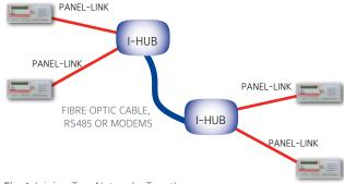
Fig 4 Joining Two Networks Together
