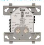
The ADM130-Mk2 is an addressable input module that allows the connection of hard contact detection devices. The module's two wire input is supervised for faults. An LED indicator allows visual monitoring of the module's status. An output is provided for connection to a remote LED indicator. Suitable remote indicators allow visual indication of the module's alarm status
