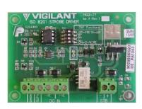
The ISO 8201 Strobe Driver generates an ISO 8201 compliant "T3" pattern for the Multi-Candela strobe 4906-9104. It connects directly to a supervised relay output of a fire alarm panel and drives one or more lines of strobes with a synchronised T3 pattern. The fire alarm panel's output supervision supervises the wiring from the panel to the strobes. The output signals of up to 5 modules can be synchronised. Four standoffs are supplied for mounting.
