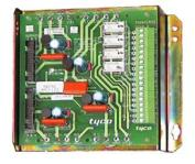
PA0792 TRAN9705-2 4x25W Transformer Module c/w Relays
