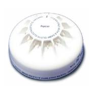
Where environmental conditions rule out the use of smoke detectors, MD601Ex/MD611Ex heat detectors may provide an acceptable, though less sensitive, alternative. For general use (particularly where the ambient temperature may be low) a 'Rate-of-Rise' (ROR) heat sensor is preferred. These detectors react to abnormally high rates of change of temperature and provide the fastest response over a wide range of ambient temperatures.
