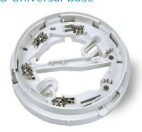
The 4B Universal Base contains no electronics and is suitable for indoor applications of the 614 series conventional (non-addressable), 814 and 850 series analogue addressable detectors. It provides excellent space for cable access and terminations. It features remote LED connections and an anti-tamper facility. The 4B base is designed to snap-fit into the ceiling tile adaptor, or screw fix to the ceiling in the traditional manner.
