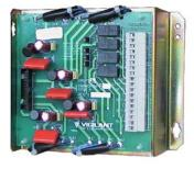
PA0796 TRAN9706-2 4x10W Transformer Module c/w Relays
