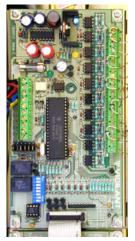
FP1068 FIB8910 FIP/BGA Master Module DD0084 FIP EOL Zener Diode
