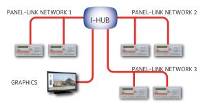
Fig 2 Joining Multiple Networks
