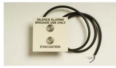
MEO433 consists of a set of (Trial) Evacuation and Silence Alarms 2-pole 2-way Bulgin keyswitches, pre-assembled and wired on a labelled White (Titania) plate. Both of these switches have their key removable in one position only to comply with NZS 4512:2003. The unit is designed to directly replace the MCP blanking plate in the standard 15U MX4428 configuration, but could also be used in other cabinet configurations, or be mounted directly to an index.
