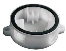
The 4B-DHM Deckhead Mounting can be used with Tyco 850 Series detectors using a 4B base. It provides an IP55 seal between the mounting surface and the detector base for superior environmental protection. The housing has four 20/25mm cable breakouts. The mounting surface should be flat over the area of the underside of the housing to ensure a stable fixing and strong enough to take the weight of the mounting, detector base and detector.
