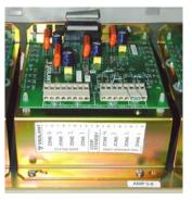
PA0795 TRAN9706-1 4x10W Transformer Module without Relays
