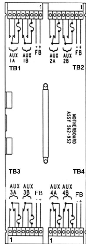
Figure 16. Wiring Connections for 4100/4120-3002 and 4100-3202 Relay Modules
