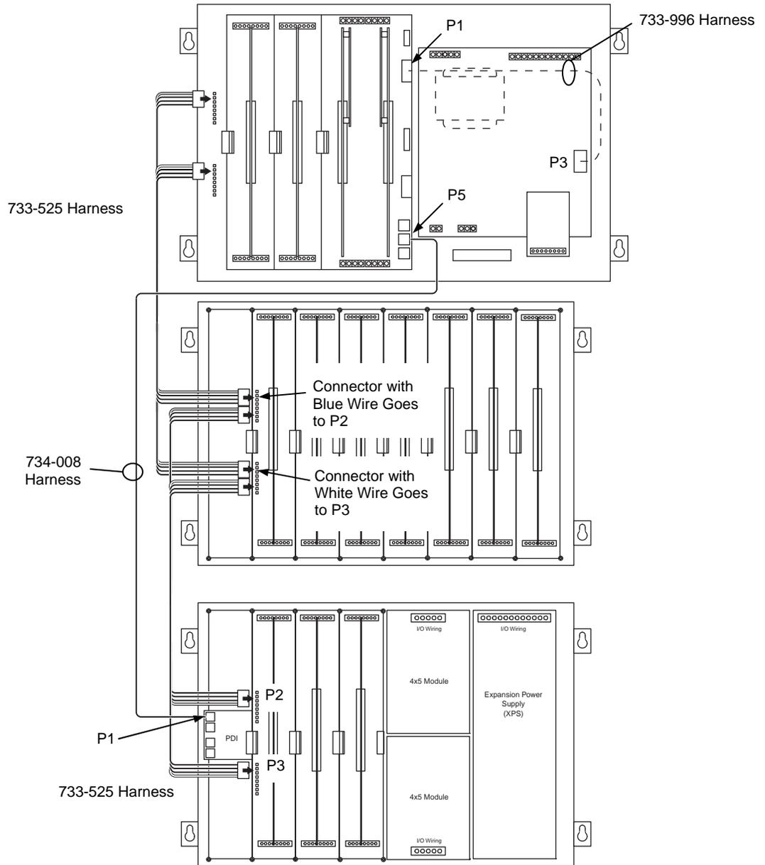
**Figure 9. Power and Communication Wiring for Motherboard (4100U/4100ES)**
