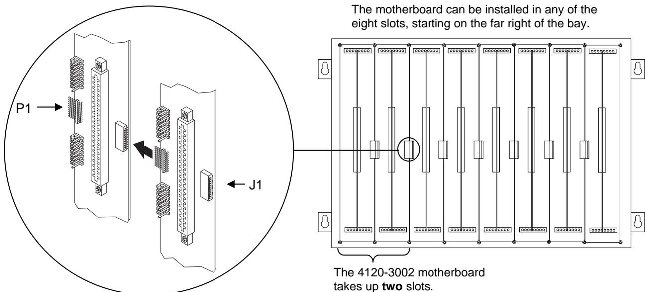
**Figure 3. Installing the Motherboard into a 4100 Expansion Bay**
