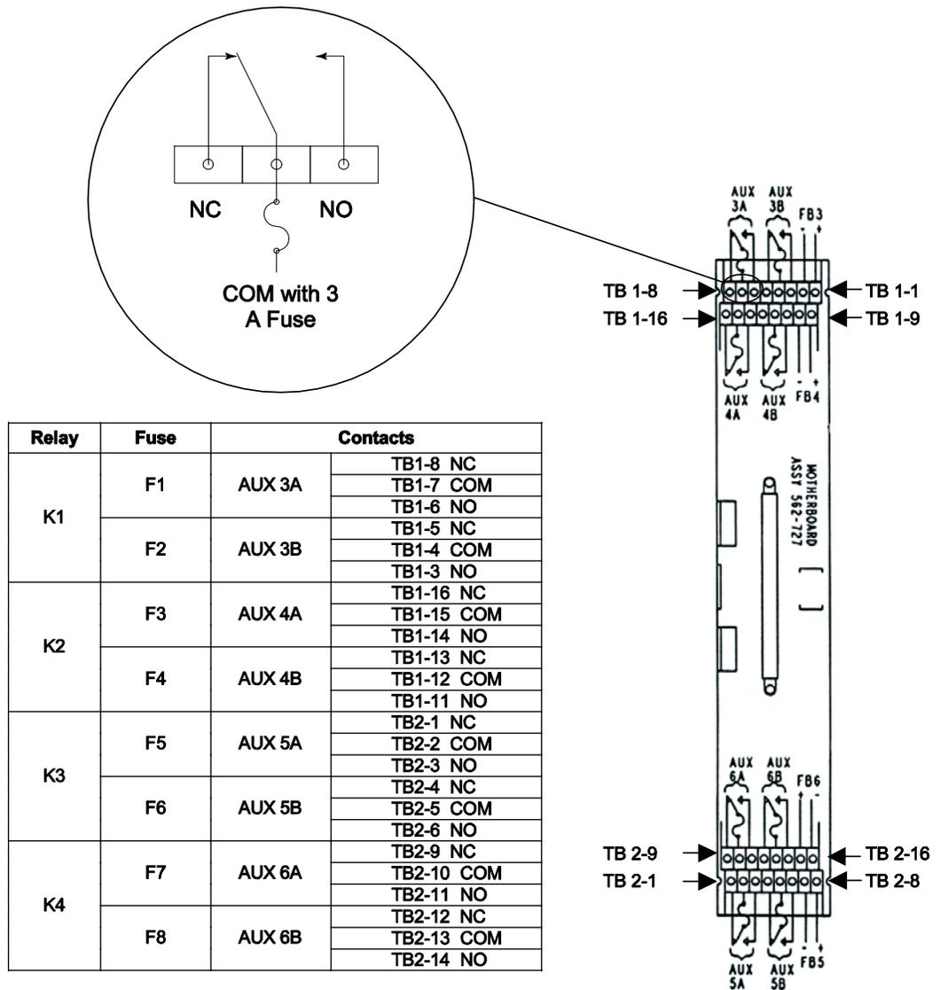
Figure 15. Wiring Connections for 4100/4120-3001 and 4100-3201 Relay Modules
