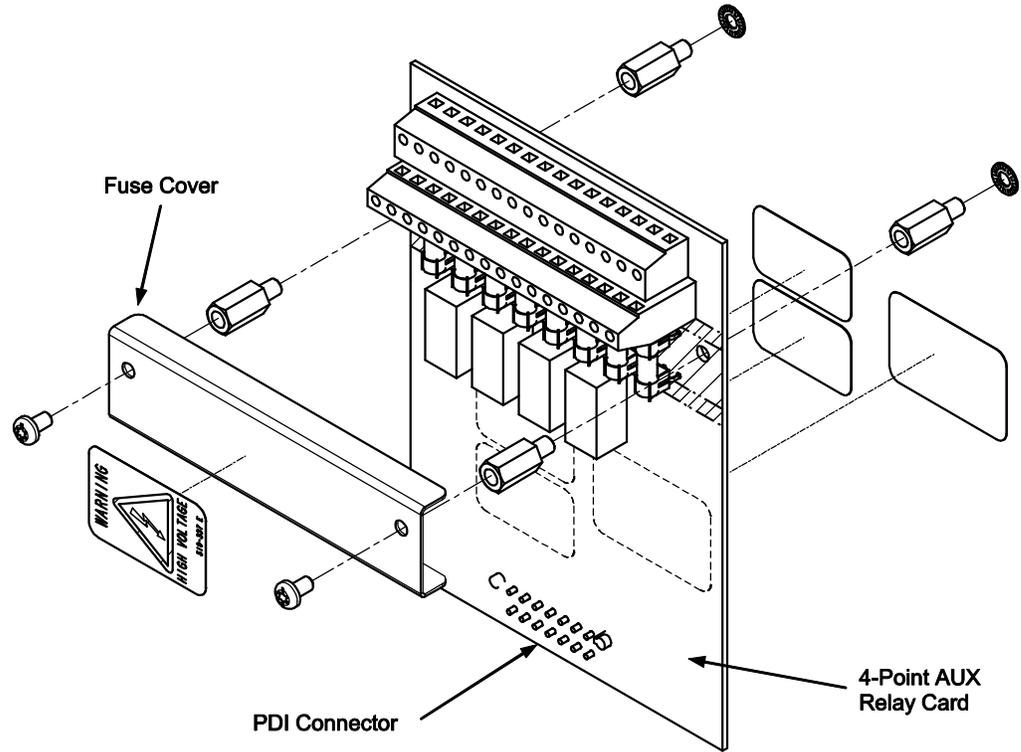
**Figure 4. 4010-9908 4-Point AUX Relay Card**
