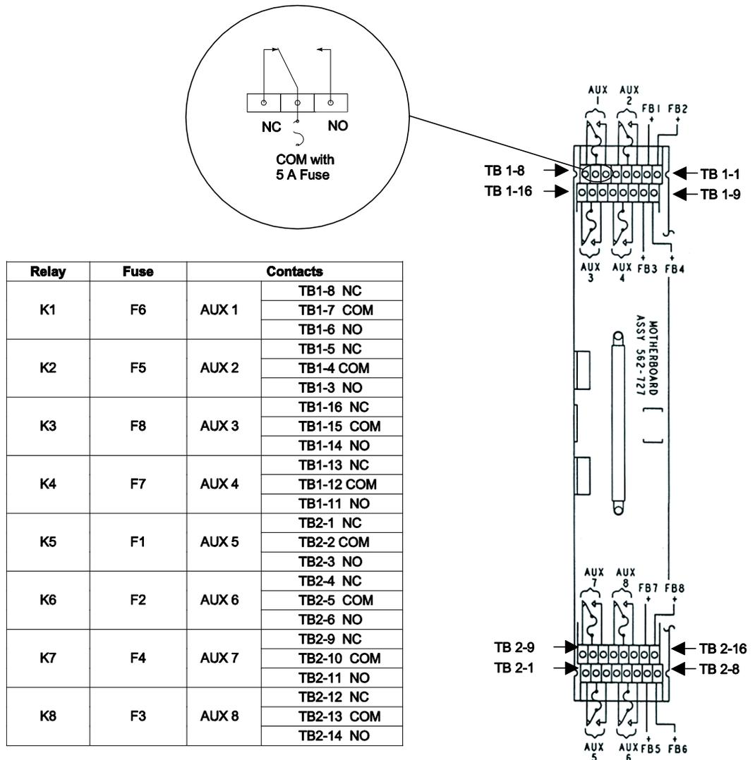
Figure 17. Wiring Connections for 4100/4120-3003 and 4100-3203 Relay Modules
