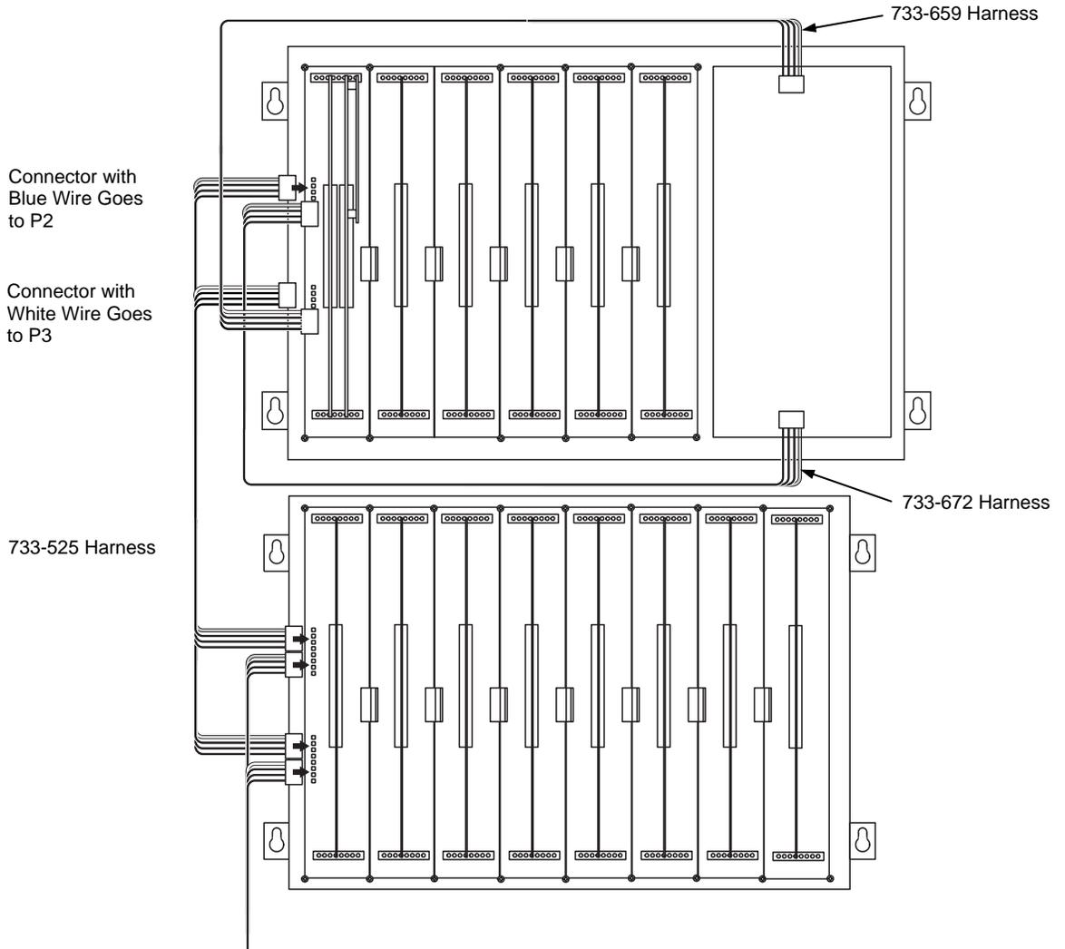
**Figure 4. Power and Communication Wiring for Motherboards (4100)**
