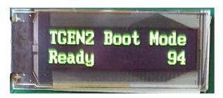
Also, the T-Gen2 will automatically enter Boot Mode on start up, if it does not have a valid firmware file contained in its flash memory.
