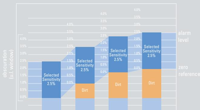
MX sensors are engineered to maintain their present levels of sensitivity. As dirt accumulates, the sensors self-adjust, notifying operators of Almost Dirty, Dirty and Excessively Dirty conditions long before they trigger a nuisance alarm. This lets you schedule maintenance on both Dirty and Almost-Dirty sensors at the same time, minimising your facility costs.
