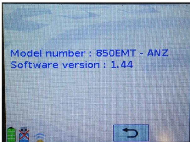
The model number must end in '- ANZ'. If it does **not** then the 850EMT has lost its Australia / New Zealand market programming and will likely exhibit the licensing problem of V1.40 described below. Such units should be returned for repair as described in the section '850EMT Units Already Exhibiting the Licensing Problem' below.
