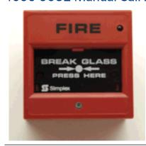
The 4099-9032 addressable manual call point provides a means to manually initiate a fire alarm condition to the 4100U c.i.e. via the IDNet channel. The IDNet channel provides the communication link between a call point and 4100U and powers the entire circuitry. Activation of the Simplex 4099-9032 manual call point requires the frangible element to be broken which causes contacts on a microswitch to close, initiating an alarm condition. Call Point reset requires the fitment of a
