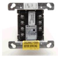
The 4090-9118 with T-Sense allows a 4100U IDNet communication channel to monitor two input contact closures with one point and control an output relay with the other point. Power is supplied from the IDNet communications channel, eliminating the need for separate power wiring. The input circuit and relay operation are controlled independently and may be disabled separately. Point association is determined at the 4100U with the device address designated as a single hardware location.
