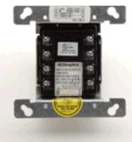
The 4090-9101 Monitor ZAMs allow a single addressable point to monitor a collective initiating device circuit (IDC) zone populated with 2-wire or 4-wire initiating devices. One IDNet address is required per device. Up to 20 collective heat and smoke detectors can be monitored by a 4090-9101 Monitor ZAM.
