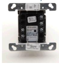
Simplex IDNet Relay IAMs allow the c.i.e. to control a remotely located Form "C" Relay contact using IDNet addressable communications for both data and module power. Typical applications would be for switching local power for control functions such as magnetic door holders, or control of HVAC components, pressurization fans, dampers, etc. Relay status is also communicated requiring only one device address.
