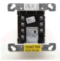
The 4090-9119 allows a 4100U IDNet communication channel to monitor an unsupervised input contact with one point and control an output relay with the other point. The module requires a single address. The input circuit and relay operation are controlled independently and may be disabled separately. At the 4100U host display, the device address is designated as a single hardware location. The individual points are considered "sub-points".
