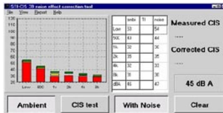
Figure 10. Ambient noise measurement
