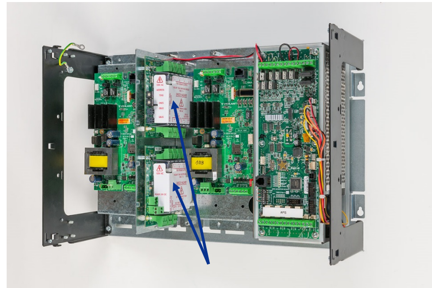
FP1120 with 2 x Splitters mounted in Simplex 4100ES PDI bay
