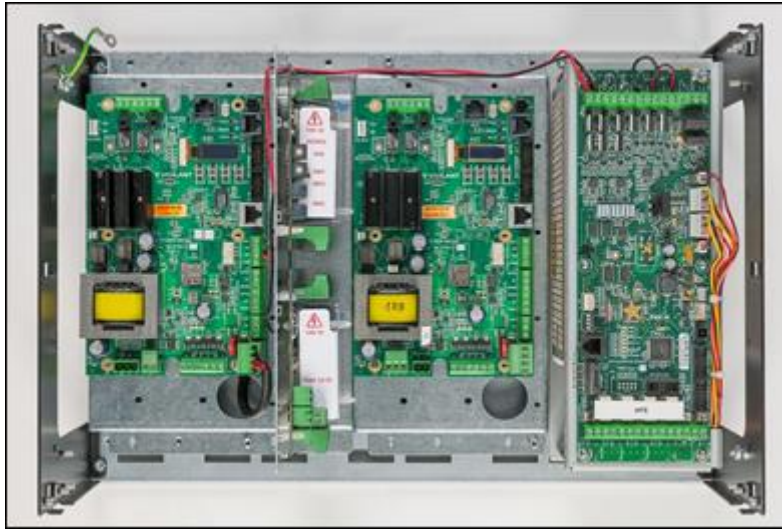
Fig 2.2 Mounting T-Gen2 in 4100ESi with APS and 100V Modules
