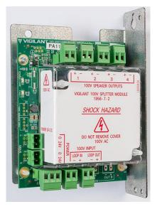
It needs to be provided with 24Vdc and the source 100V signal, which can be daisychained on to multiple modules using the loop-in/loop-out terminals.
