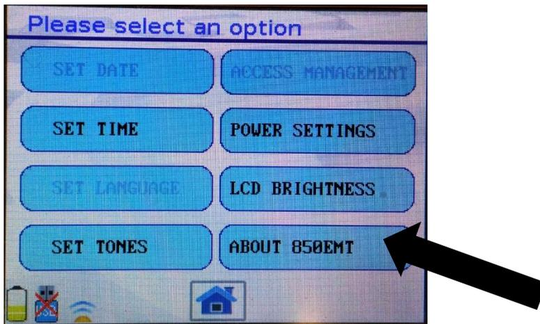
3. A screen should then come up showing the version number of the firmware installed on the 850EMT unit:
