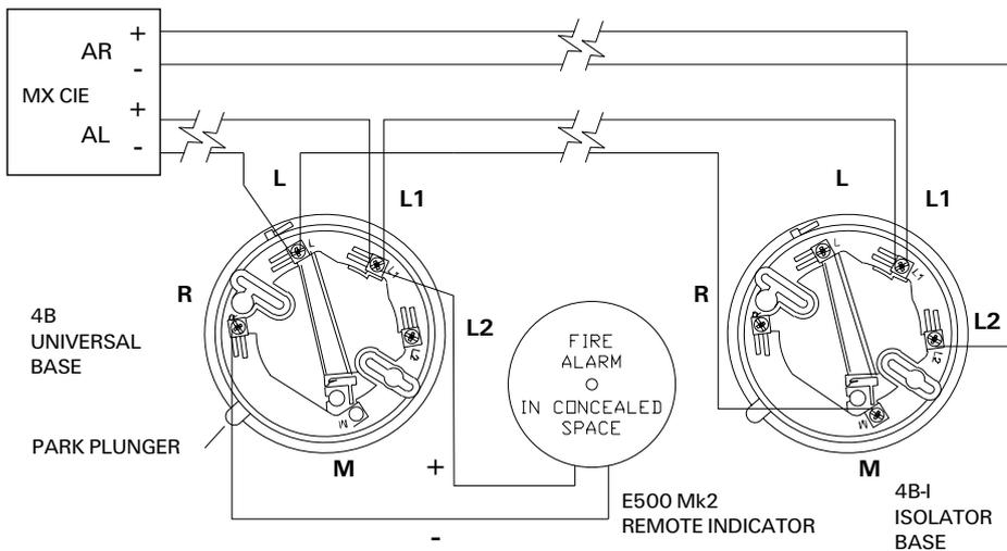
The MX CIE can be programmed to illuminate a Remote Indicator for detectors in alarm other than the detector base to which the Indicator is connected.
