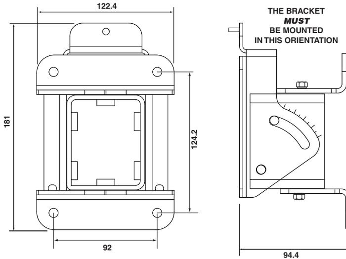
**Fig. 12 Adjustable Mounting Bracket and Surface Mounting Dimensions**
