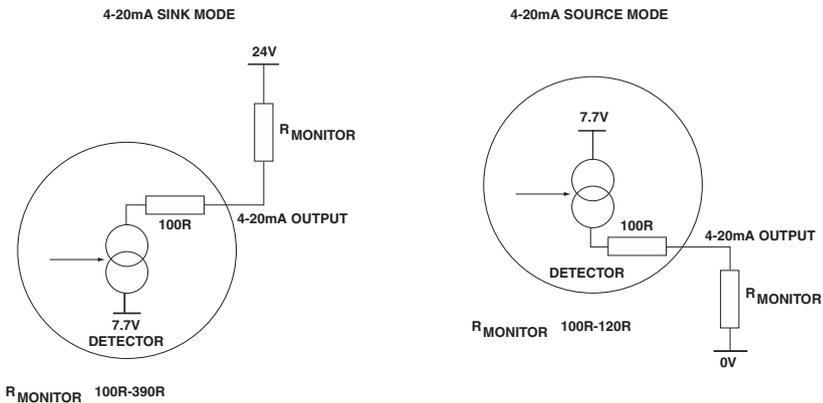
**Fig. 7 4-20mA Current Sink/Source Wiring Diagrams**
