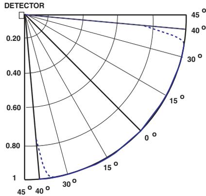
**Fig. 20 Relative Range vs Angle of Incidence - Vertical Plane**
