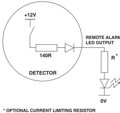
**Fig. 10 Remote LED Wiring Diagram**
