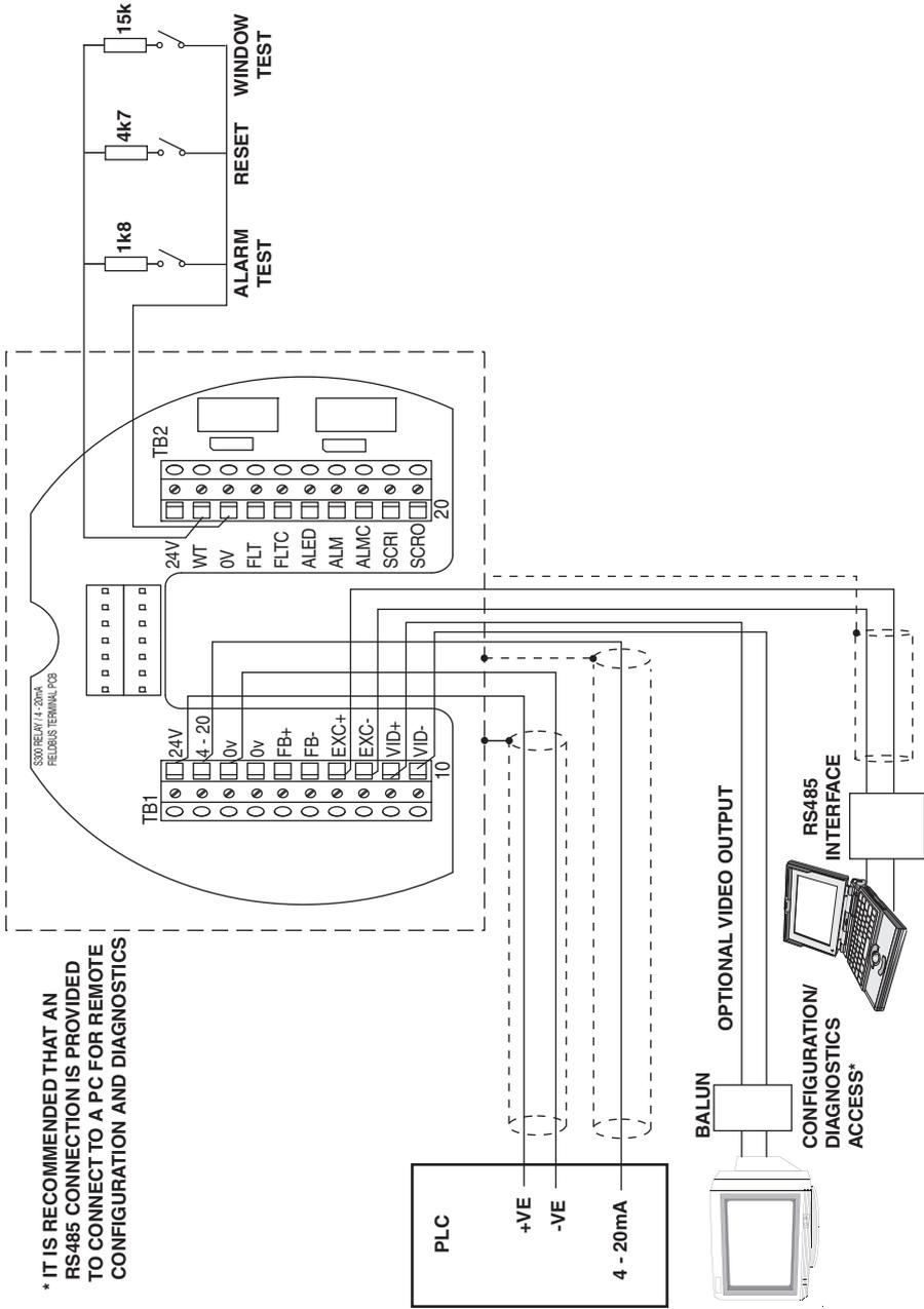
Fig. 26 4-20mA Output Wiring Diagram
