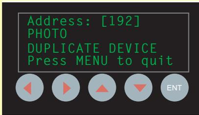
To troubleshoot duplicates, go to the TSIT Error or Duplicate menu and send a command to the device address to activate the device's LED. The devices set to the displayed address will have their LEDs lit as long as TSIT displays their address. In the example shown, any devices with LEDs at address 192 would
