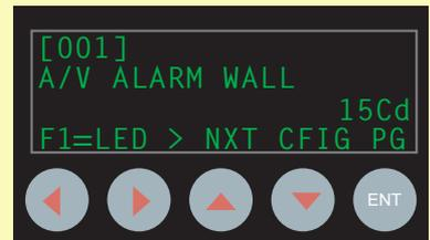
The image to the right shows information that can be displayed after executing "IDNAC Test". The device address is displayed in brackets. Beneath, the device type info indicates this is a Wall
