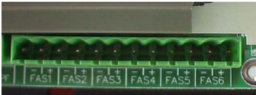
Figure 2 – Six fire alarm systems can be connected to the ASE
