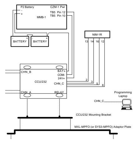
The CCU/232 is designed to mount on the MXL-MPFO adaptor plate for the MOM-4 position, occupying one D2300CP position (MXL Only). CCU/232 can also mount to SYS3-MPFO adaptor plate for System 3 enclosure (EA-31, EA-32, EA-35) mounting.
