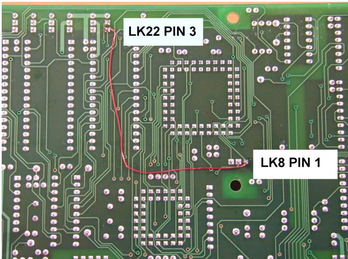
**Photograph 1 - Fitting Wire Link to Rev 2&3 1931-111 Iss B Controllers**
