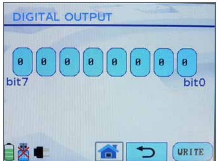
Fig. 19: Test Digital Outputs Screen
