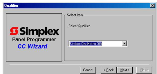
This equation stops the horn but keeps the strobes going.
